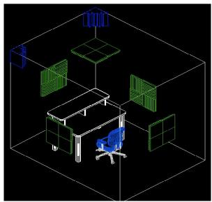
The pattern shown in this rendering is only one example of the way that the panels and bass traps of your Saturn 1 kit can be oriented in the room. If you desire a different aesthetic pattern, you can rotate the panels however you like as long as the guidelines listed above are followed as this will not detract from the performance of the acoustic treatment. Universal Acoustics foam materials will not only dramatically improve your acoustics but can also make your workspace look great.
